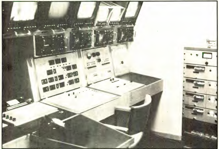
This station in Adelaide, South Australia, was the first successful attempt (1965) to automate a complete TV programming facility. It featured an automatic program controller with magnetic drum memory, permitting mechanical schedule preparation, automatic all day switching and machine control, and as a consequence, mechanical billing, accounting and reporting.
